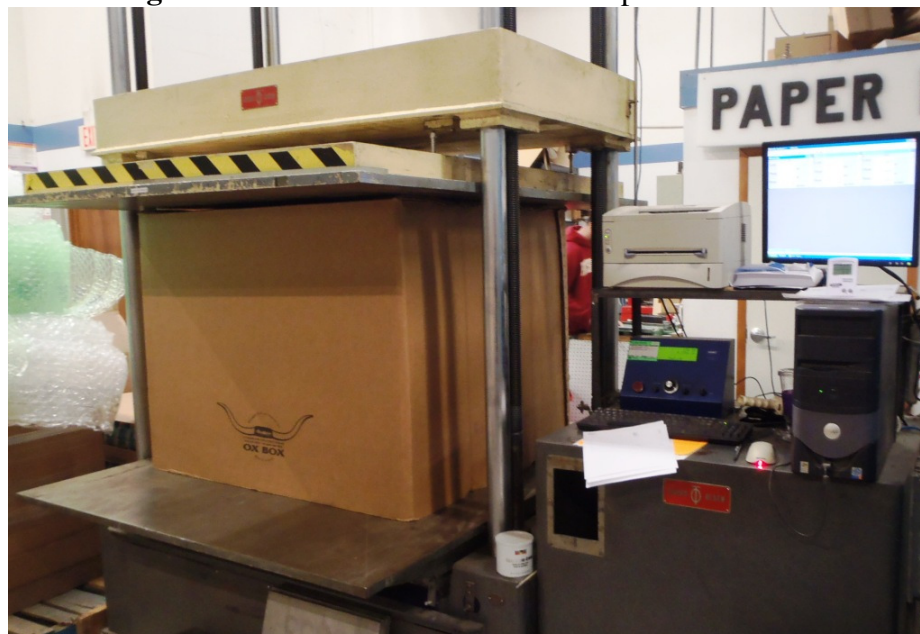
Figure 1. Modified Tinius-Olsen Compression Tester
